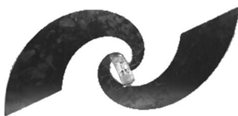
Fig 2.5. A typical wideband spiral antenna.
