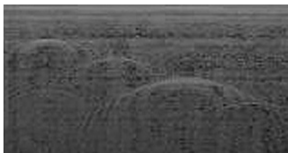
Fig 1.3. B-scans of several objects above the ground using a SF-GPR (SAR) with double ridged horn antennas. The hyperbolic shapes are the result of averaged pulses over a synthetic aperture.
